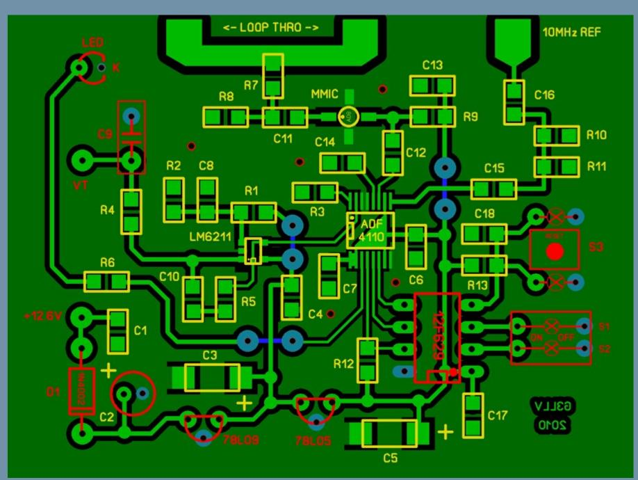
The double-sided PCB layout seen from above with the YELLOW SMD and GREEN track layers underneath. The RED through-hole components and BLUE pads/links are on top together with five small RED circles indicating riveted vias. Pin-8 of the 12F629 is soldered on both sides of the board. A viewer and print utility for this layout is available on the "Software" page.
