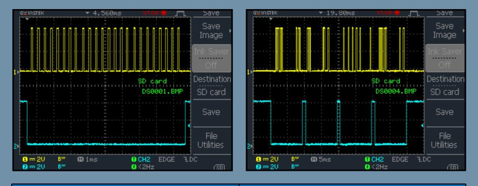
The CLK and LE waveforms for each EEPROM-to-latch load. The DATA and four LE waveforms for a complete EEPROM block read.
